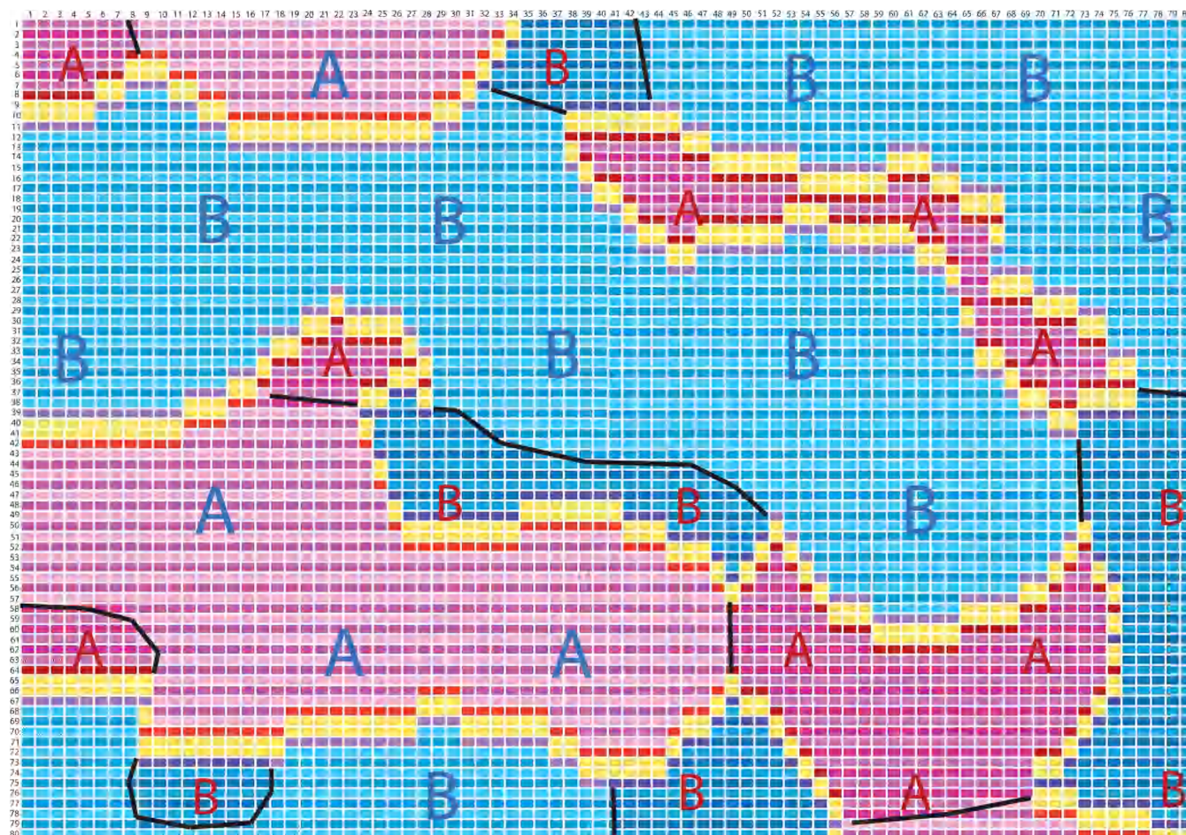
Figure 7. (c) All disordered regions eliminated except for two ordered blocks required along (001) of every antiphase domain boundary. Synphase boundaries marked in black occur where small A regions postulated to be enriched in Fe (note darker red shades) are in contact with larger A regions (or vice versa). Antiphase boundaries are decorated with both red and violet contact layers and two yellow disordered layers.
