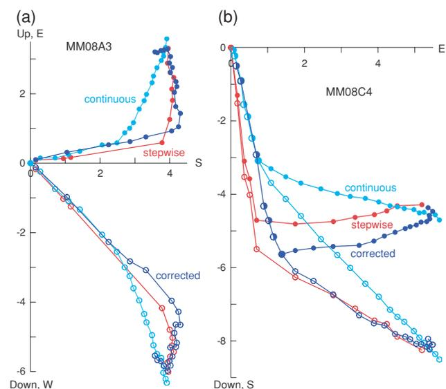
**Figure 1.** Results of stepwise and continuous thermal demagnetization of a bivectorial remanence in two samples of the Milton Monzonite, displayed on orthogonal vector diagrams (data: Schmidt & Clark 1985). Open and filled points are vertical- and horizontal-plane projections, respectively. Agreement is poor between the stepwise and untreated continuous data for the lower- $T$  partial TRM but becomes quite close when the continuous data are corrected by dividing each result by  $M_S(T)$ .
