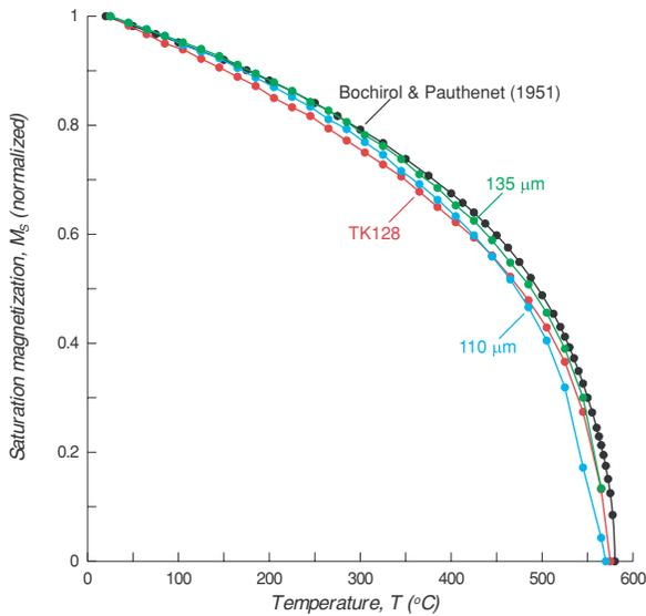
**Figure 3.** Magnetization measured in a 0.5-T field as a function of temperature  $T$  for sister samples of those used in pTRM experiments. The results, all resembling the standard  $M_S(T)$  curve of magnetite (Bochirol & Pauthenet 1951), were used to convert continuous thermal demagnetization data to equivalent room-temperature values.
