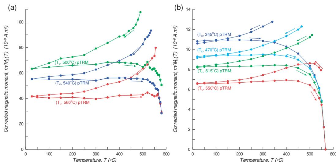
**Figure 7.** Zero-field cycling of various pTRMs in the style of Fig. 2 for (a) the 110  $\mu\text{m}$  magnetite samples and (b) the TK49 minicore. Corrected to room-temperature values, pTRM intensities decrease with cooling, although not as markedly as in Fig. 2. However, on heating, the curves are almost flat and recovery of pTRM intensity is minimal, in contrast to the Fig. 2 results.
