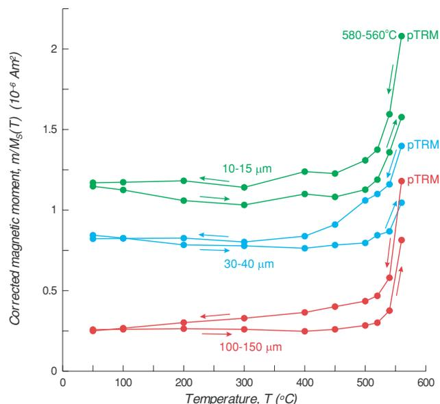
**Figure 2.** Zero-field cycling of pTRM (580 °C, 560 °C) from 560 °C → 20 °C → 560 °C for magnetite samples of various grain sizes (data: McClelland & Sugiura 1987). Moments have been corrected to equivalent room-temperature values by dividing each result by  $M_S(T)$ . Each pTRM decreases sharply on cooling below 560 °C but recovers part of its intensity in heating back to 560 °C.
