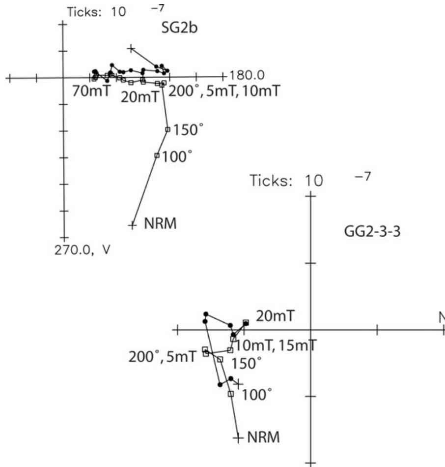
**Figure 3.** Representative vector endpoint diagrams showing demagnetization behaviour during low-temperature thermal demagnetization followed by alternating field demagnetization. The State Gamelands locality (sample SG2b) gave the best results. The Glenshaw Glass locality (sample GG2-3-3) gave some of the poorer quality demagnetograms.
