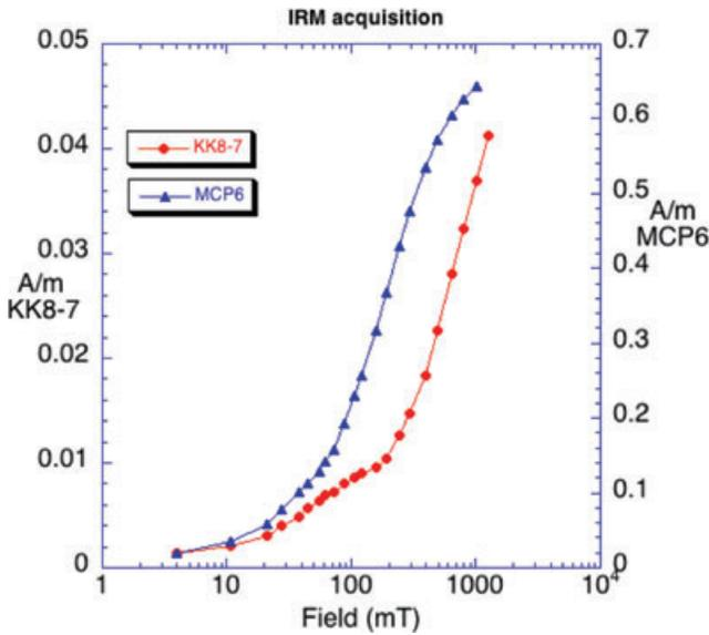
**Figure 2.** IRM acquisition results for magnetic extracts from the Mauch Chunk Formation (MCP6) and the Kapusaliang Formation (KK8-7). Note a break in slope in both curves at about 100 mT indicating both low coercivity magnetite and high coercivity haematite in these magnetic extracts.
