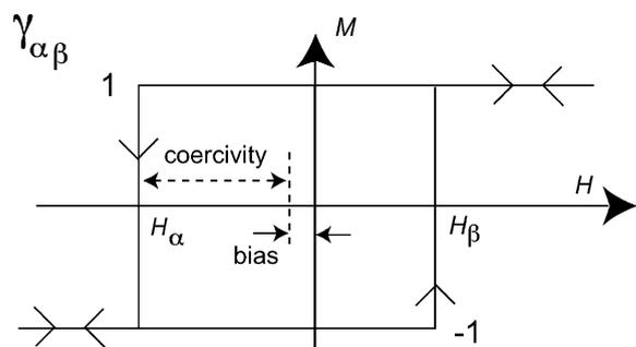
Fig. 3. The hysteron  $\gamma_{\alpha\beta}$  equals 1 for large values of  $H$ , switches to  $-1$  when  $H$  falls below  $H_\alpha$  and remains at  $-1$  until  $H$  rises above  $H_\beta$ . The half-width of the hysteron is its coercivity, and the horizontal offset of its centre is its bias.
