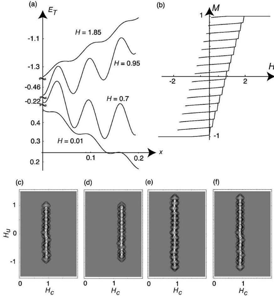
Fig. 8. (a) Total energy as a function of DW position  $x$  for various applied fields  $H$  calculated with sinusoidal DW energy in Eq. (5) for  $E_p = L = N = 1$ . The curly lines on the vertical axis represent breaks where the scale has been changed to emphasise the features on each curve. (b) A set of calculated FORCs for  $E_p = L = N = 1$ . Calculated FORC diagrams for (c)  $E_p = L = N = 1$ ; (d)  $E_p = 1.4$ ; (e)  $N = 1.3$ ; and (f)  $L = 1.3$ .
