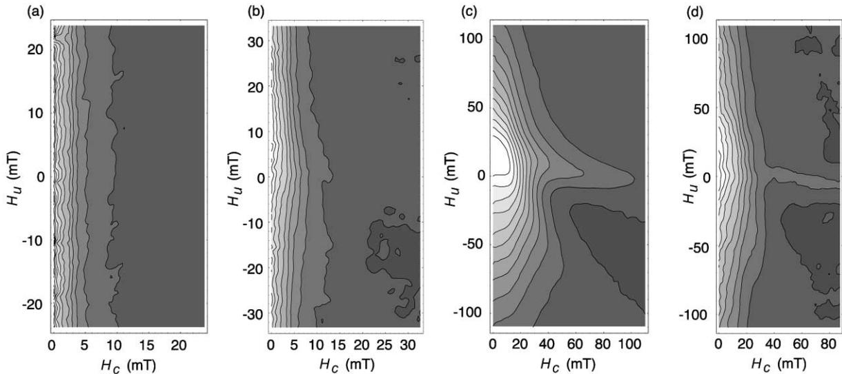
Fig. 6. FORC diagrams ( $SF = 3$ ) for (a) a sample of M80 transformer steel; (b) a 2 mm grain of magnetite, after annealing; (c) the same 2 mm grain of magnetite before annealing; and (d) a 125  $\mu\text{m}$  magnetite grain (no annealing) from sample HM4 (see Hartstra, 1982).
