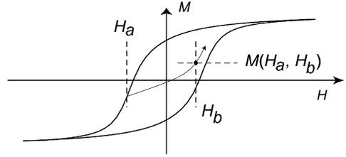
Fig. 1. Example of a major hysteresis loop with reversal point at  $H_a$ . FORC is the curve that starts at  $H_a$  and proceeds back to positive saturation. A magnetisation at an applied field  $H_b$  on the FORC with reversal field  $H_a$  is represented by  $M(H_a, H_b)$ .
