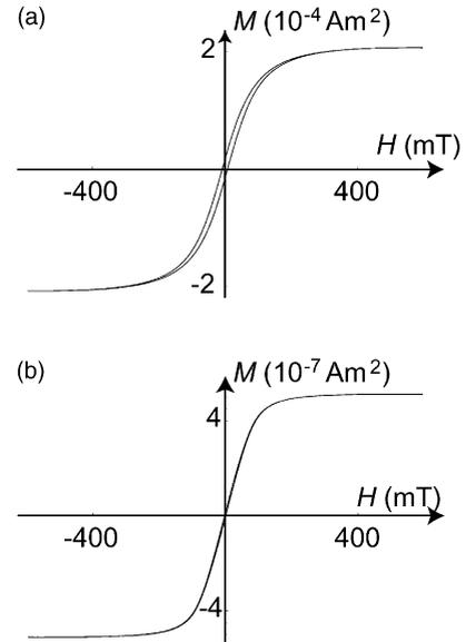
Fig. 5. Major hysteresis loops for two of the analysed samples: (a) a 2 mm magnetite grain before annealing; and (b) a  $125\ \mu\text{m}$  magnetite grain. On this scale, the loop in (b) appears to be closed. Hysteresis parameters for these samples are given in the text.
