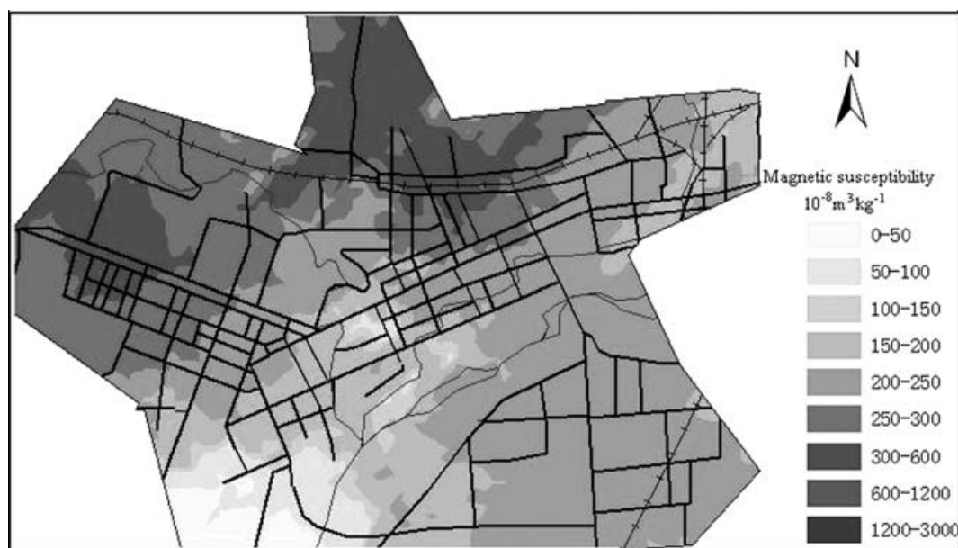
Figure 3. Map of magnetic susceptibility ( \times 10^{-8} \text{ m}^3 \text{ kg}^{-1} ) distribution, created using ArcGIS, for the urban topsoils in Luoyang City.
