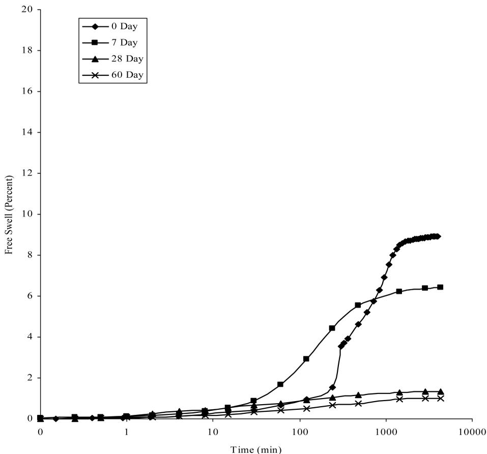
**Figure 4.** Free Swell versus Time for 18% Initial Moisture Content (IMC) and 20% Bentonite at each Curing Period.
