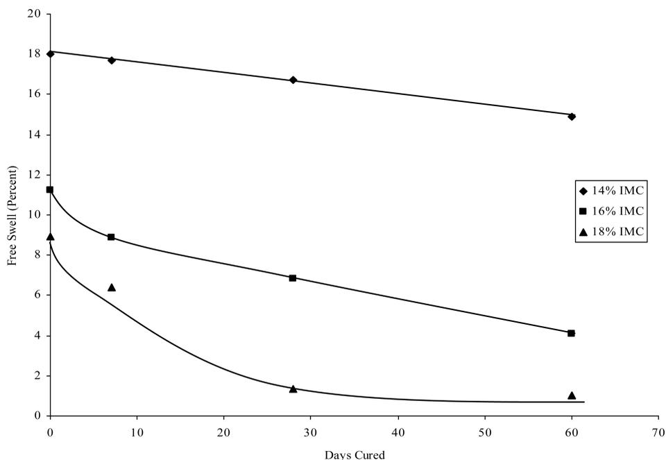
**Figure 5.** Maximum Free Swell Response with Curing Period for 20% Bentonite Specimens.
