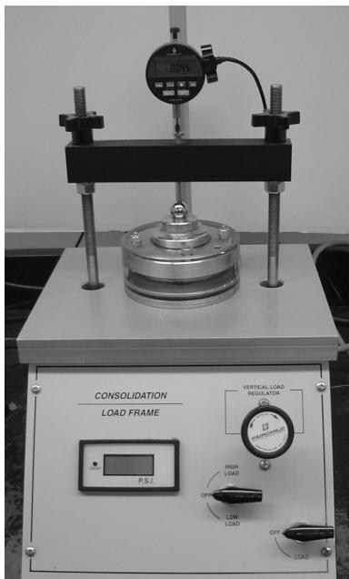
**Figure 1.** Free Swell Test in Progress.
