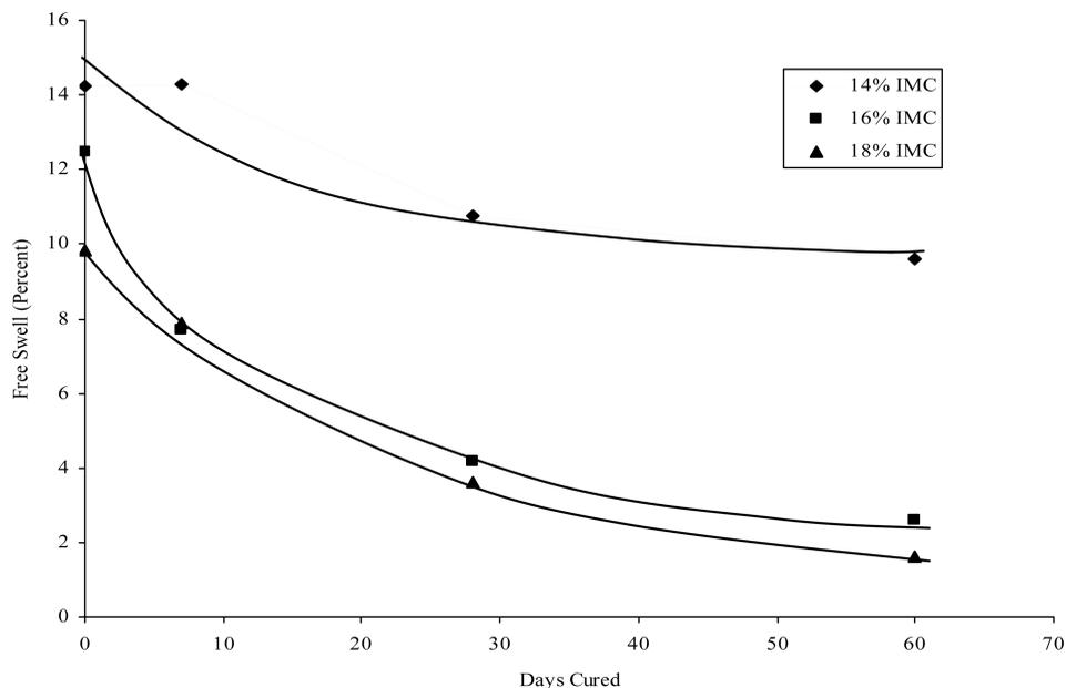
**Figure 6.** Maximum Free Swell Response with Curing Period for 15% Bentonite Specimens.
