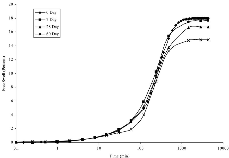
**Figure 2.** Free Swell versus Time for 14% Initial Moisture Content (IMC) and 20% Bentonite at each Curing Period.
