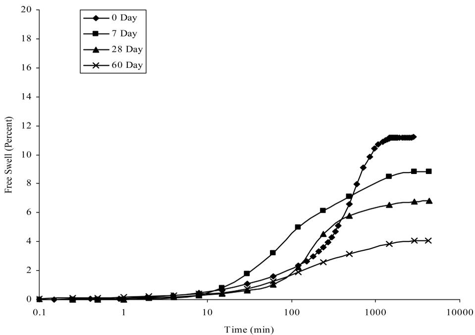
**Figure 3.** Free Swell versus Time for 16% Initial Moisture Content (IMC) and 20% Bentonite at each Curing Period.
