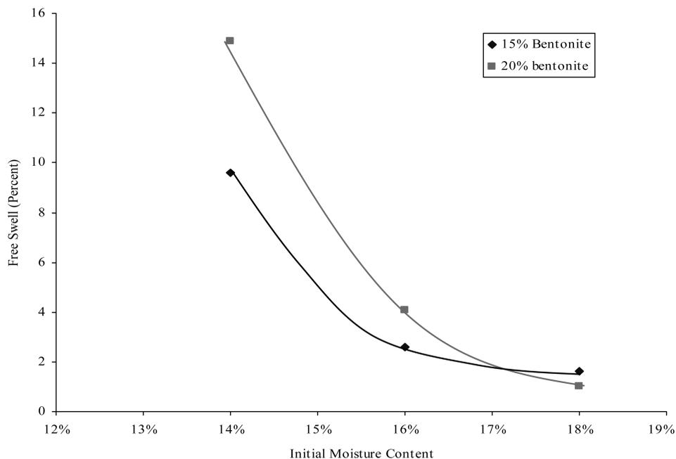
**Figure 7.** Maximum Free Swell Response with Initial Moisture Content after 60 Days of Curing.
