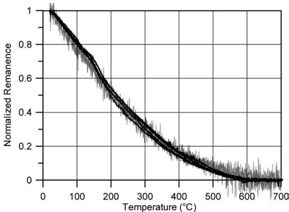
**Figure 5.** Thermomagnetic curves for the six El Cristo samples ( $\times$  in Fig. 2) and for the Mar del Plata ash sample. Because they are essentially indistinguishable, all but one of the curves are indicated in black. The data for the weak sample from 920 cm depth is shown in grey to allow the reader to appreciate the fact that, despite its low signal-to-noise ratio, it too has the same shape as the others.
